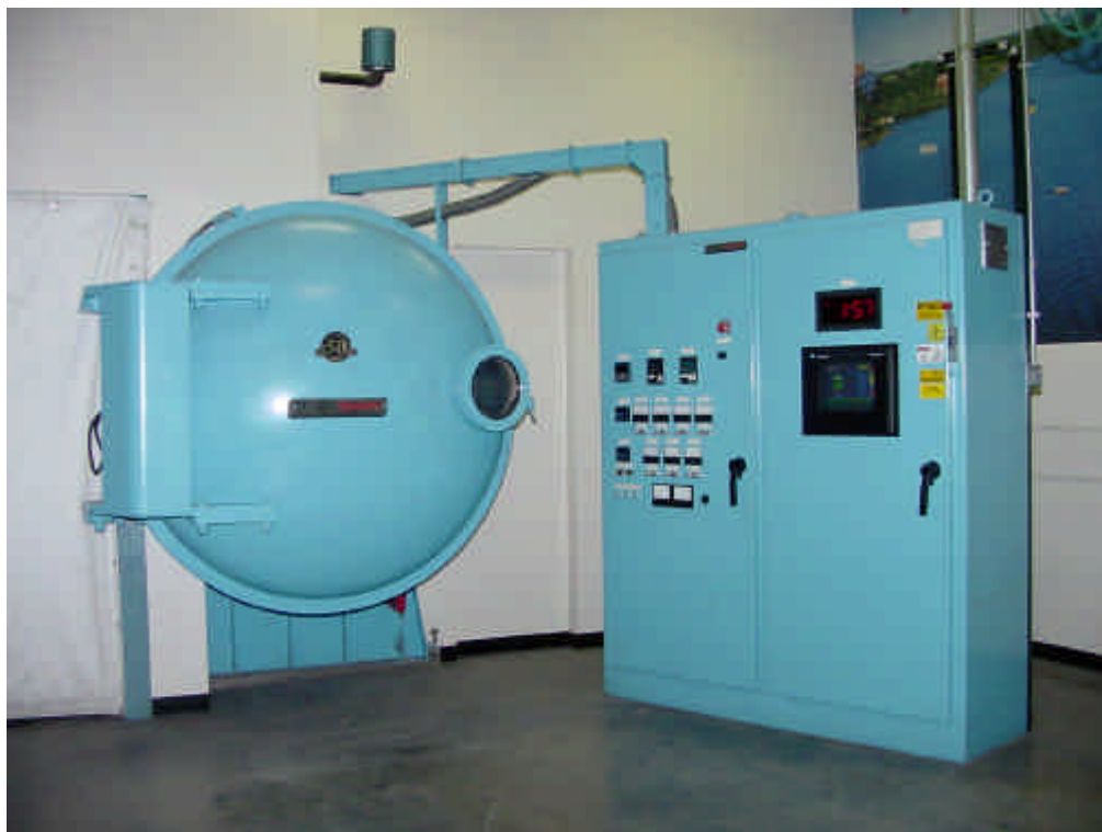
Figure 1. Extended Length IVD Aluminum Coater at Boeing – St. Louis
